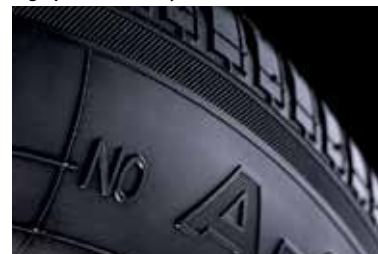
The "NO" mark engraved on the sidewall expresses Porsche approval.
